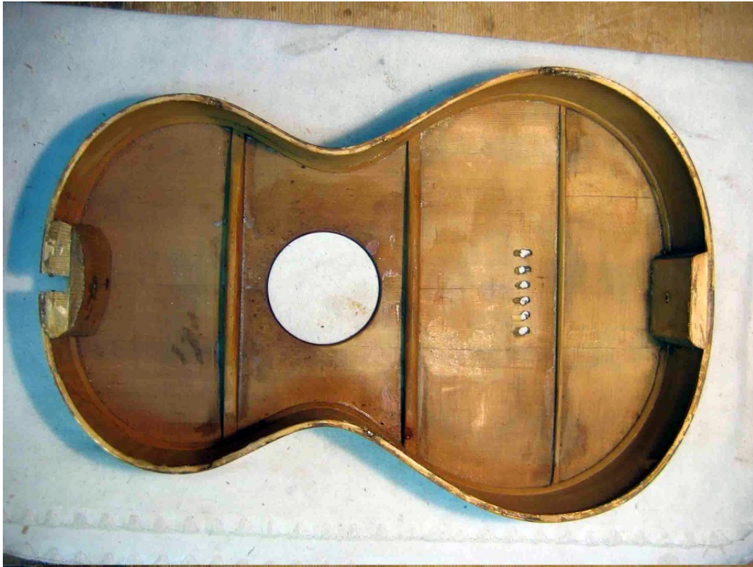
Ladder-bracing on an A. Stauffer & Comp. guitar, ca. 1825 [Bracing1]
