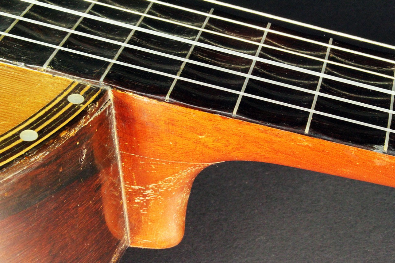
Mother-of-pearl I-type frets in a scalloped fretboard [FretsMotherOfPearl]
