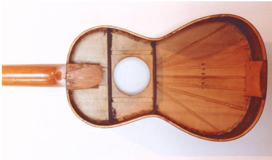
Fan-braced top of an instrument by L. Panormo, 1832 [Bracing4]
