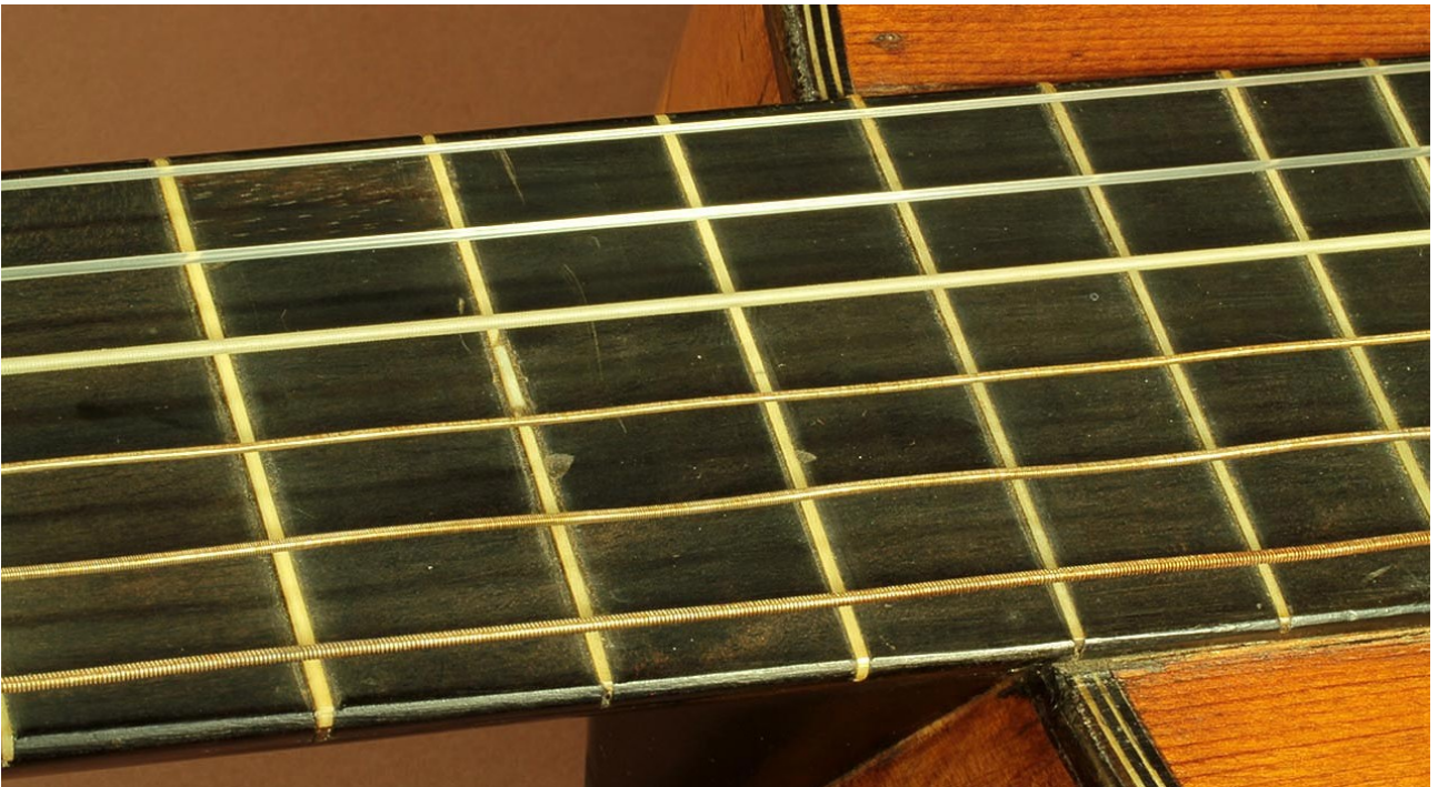
I-type frets made of bone embedded into a flat, non-scalloped fretboard [FretsIvory]
